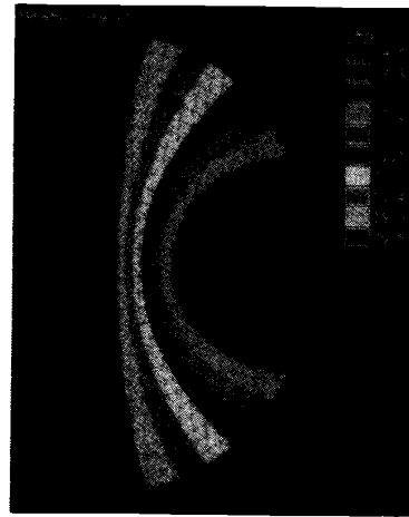
Fig. 9. Temperature profile for a laser rod with near-Gaussian deposition of 0.6 W heat load and experimentally measured boundary conditions of a 30.5°C isothermal on the flat heatsink surface and convection cooling of the curved face at an ambient air temperature of 23.8°C.
